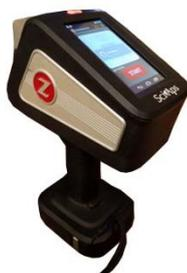
**Fig. 1. Handheld LIBS SciAps Z300 used to produce the set of calibrations to analyze spodumene and petalite from the Barroso-Alvão field.**
