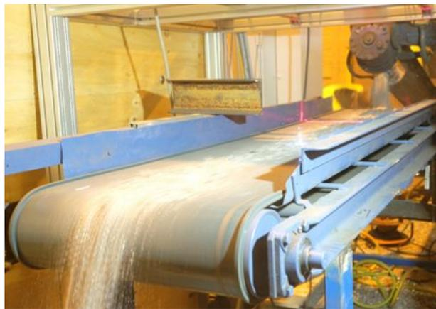
Fig. 1. Continuous flow of aluminium metal chips inspection by scanning LIBS sensor.
