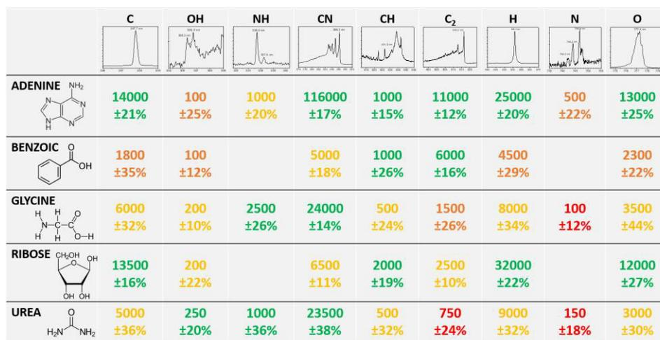
Fig. 1. Mean intensities of organic emission signals detected for each analyzed molecule in a simulated Mars atmosphere. An example type spectrum of each atomic line/molecular band is also shown.
